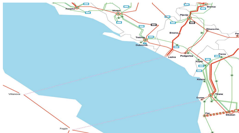
Existing and planned transmission corridors in Montenegro.
